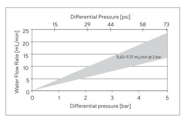
Due to the shorter fiber length in the Virosart $^{\circ}$  Media lab module, the water flow rate is 450 LMH/bar  $\pm$  25%, 25°C.
