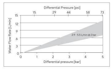
The water flow rate for the Virosart $^{\circ}$  Media mid-scale modules 0.3 m $^{2}$  is 420 LMH/bar  $\pm$  30%, 25 $^{\circ}$ C.
