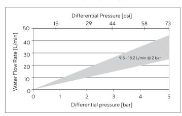
The water flow rate for the Virosart $^{\circ}$  Media process modules 1.0 m $^{\circ}$  is 420 LMH/bar  $\pm$  30%, 25 $^{\circ}$ C.
