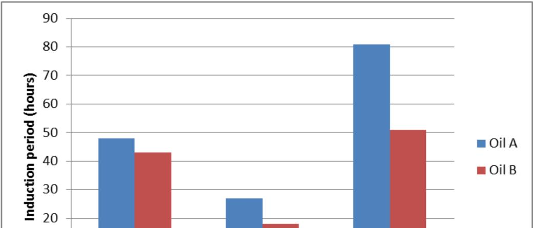
The basic principle of the Oxitest is that a weighed representative sample of product is placed in the sample chambers which are then closed. The sample chamber is pressurised with oxygen and heated to the selected temperature. Pressure drop is monitored as the sample consumes oxygen, and the induction period calculated.
