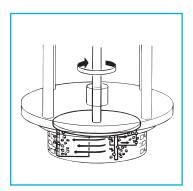
The materials are subjected to intense shear within the workhead. Any agglomerated particles are fully broken down in the clearance between the ends of the rotor blades and the stator wall.
