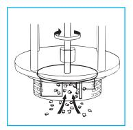
The vessel is charged with the required amount of liquor. The mixer is started and the isinglass is added. The high speed rotation of the rotors creates a powerful suction which draws water and the isinglass particles into the workhead.
