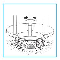
The product is forced out through the stator and projected back into the main body of the mix as fresh material is simultaneously drawn into the workhead.
