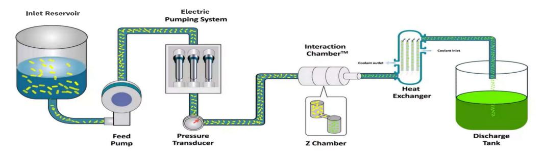
Product enters the system via the inlet reservoir and is pulled into a patented sanitary electric pumping system which pushes the material through a fixed geometry Interaction Chamber™ where it experiences consistent, high shear rates and impact forces. All material receives the same treatment to achieve repeatable, reliable results. After passing through the Interaction Chamber™, the product is cooled in the heat exchanger resulting in reduced denaturing and increased yields.
