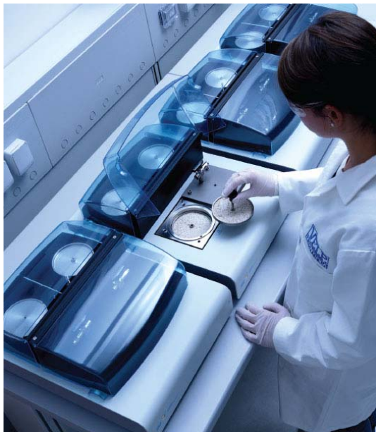
FIG. 1. Sample loading in the Oxitest chambers
