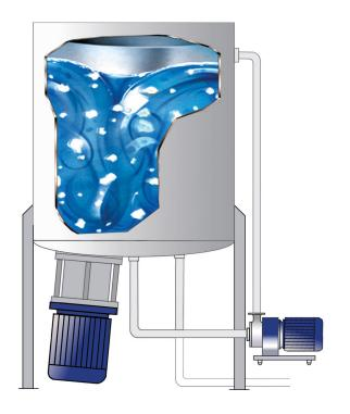
The solids are rapidly reduced to smaller pieces which are drawn into the interior of the workhead and subjected to intense shear before being forced out through the stator and back into the surrounding liquid.
